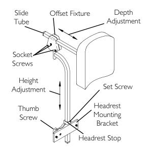
FIGURE 9.1 Removing/Installing/Adjusting Headrest
